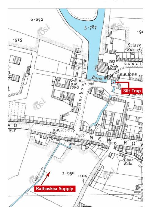
The Rathaskea Feeder Supply flows into the eastern terminus of Naas Harbour. It appears that the natural line of the stream was followed allowing it to turn at 90° before entering the Harbour, thus slowing the water with the intention of trapping silt. Otherwise the feeder could have been piped under New Row and run direct beneath Harbour View to the Harbour.
